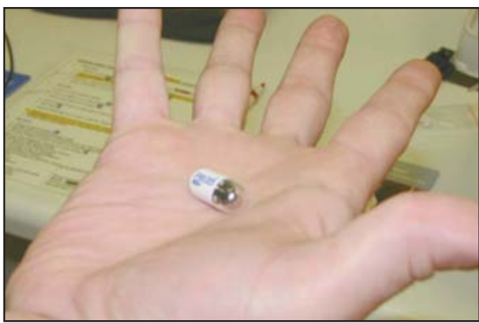
The Pill Cam is the first device capable of providing doctors with images covering the entire 21 feet of the small intestine.
